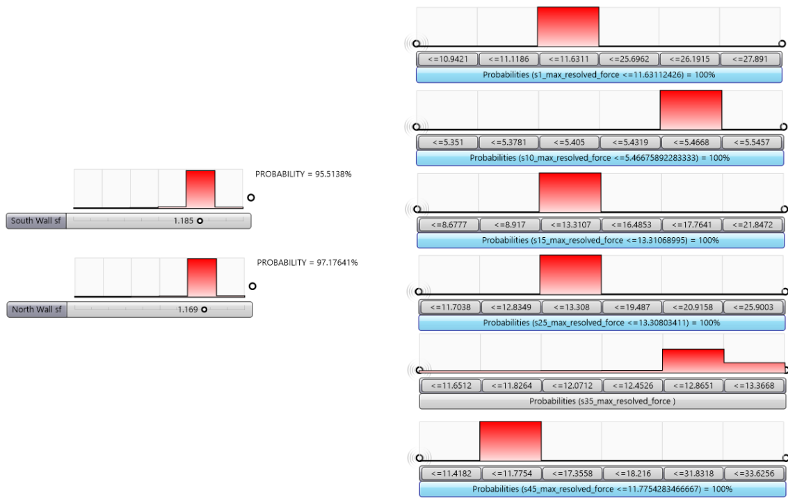
Figure 6.29: Probability (s1, s10, s15, s25, s45_max_resolved_force \leq ~13.32kN)=100%.
